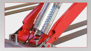
4\_ADJUSTABLE MECHANICAL SAFETY DEVICE Adjustable mechanical safety device, also for exact adjustment for wheel alignment.
