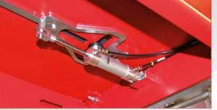
6\_SLIDING PLATES Sliding plates with air central locking.
