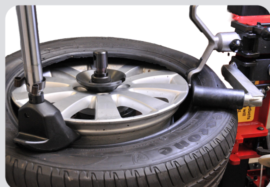
Pneumatic bead pressing arm + standard pressing roller
