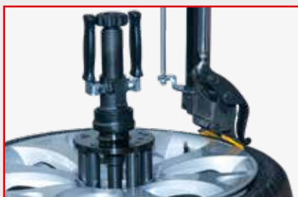
Top bead demounting procedure
